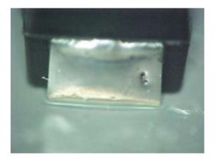
The example shows satisfactory wetting of capacitor terminations with a minor pin hole in the upper region which would not affect the joint area.
