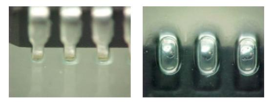
Satisfactory solder wetting on all PLCC leads after reflow test. The second PLCC sample shows a close up of the base of the leads through the glass test substrate. Figure 3 & 4.
