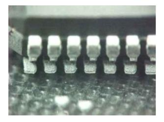
The image shows a component placed on the surface of the paste deposit previously printed on the glass slide.
