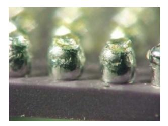
The example ceramic BGA below shows a series of high temperature balls with marginal wetting.
