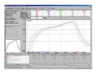
The profiles show selected positions on the board and the temperature variations across the board surface. The profiling was conducted using an ECD Mole profiling system.
