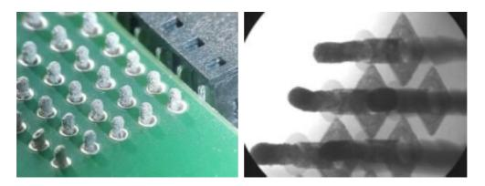
Two examples of the har-busHM+ connector after assembly and prior to reflow soldering. The first view shows the base of the board after insertion of the connector and limited paste displacement on the tips of the pins. The second view, and slightly more unusual, is the X-ray image of the board with the paste deposit visible on both sides of the board prior to reflow.
