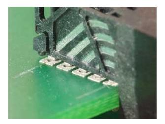
The har-busHM+ is a 110 pin row connector especially designed to minimise temperature differentials on the surface of the board during reflow and remain designed for automatic assembly
