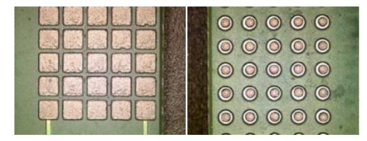
The print deposits produced maximized the surface area on the topside of the board as well as through the holes as shown on the two examples above
