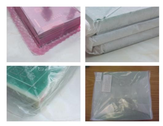
Different packaging used in the industry for printed boards, shrink wrap, tissue paper interleaved, plastic bags and combination of tissue and plastic bags
