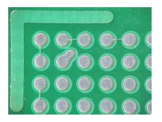
BGA pad with a wetting indicator, a little larger than necessary but it does show the wetting under xray inspection
