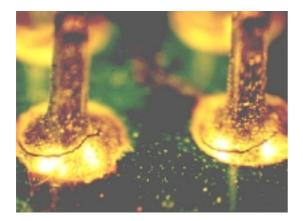
Solder joint failure due to incorrect hole to lead ratio
