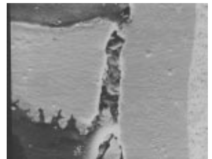
Figure 2: Inner-layer separation occurs when de-smearing, a cleaning process, is not properly conducted.
