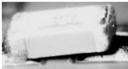
Figure 3: The component has lifted because of the thick solder mask; during reflow it acted like a fulcrum lifting the part just above the pad surface.
