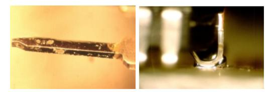
The examples show poor solderability found when moving over to no clean materials on both conventional and surface mount terminations
