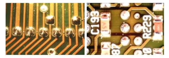
Two examples of solder balls on solder mask. One is a random ball example and one is design related
