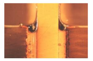
Poor soldering performance shown by this section is due to solderability of the solder finish and the performance of the liquid flux
