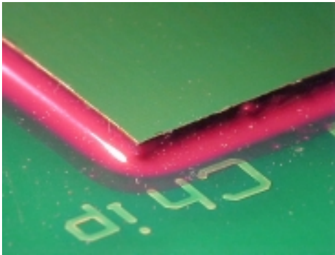
Flip chip examples produced with the same process for soldering trials with no-flow underfill and soldering and underfilling after reflow
