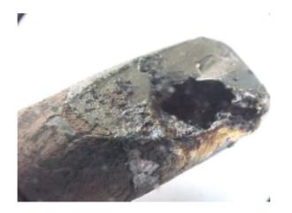
Example damage soldering iron tip and erosion of the copper under the iron plating with lead-free solders
