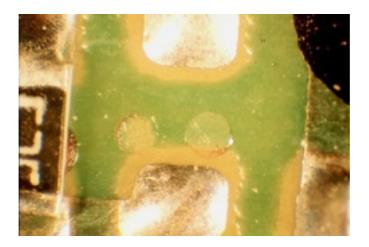
Example of component loss which is related to the adhesive's compatibility between the adhesive and the solder resist. Change in solder mask type from solvent to aqueous or degree of cure
