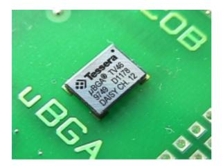
Shows a uBGA placed and reflowed in place with reference to the corner marks without vision.
