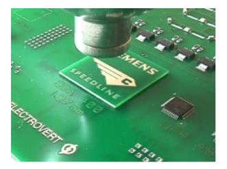
Shows a hand held IR rework tool being used to reflow all the solder joints on the BGA prior to lifting the part from the board. This type of procedure is supplemented with under board heating to approximately 120-130°C prior to applying top side heat. (image 180.jpg)
