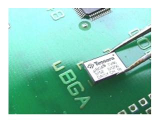
Shows the replacement of a 0.025" pitch component being manually placed with reference to the corner marks on the circuit board pattern. Corner marks are invaluable to aid the assembly operation and to assist during prototyping of BGA or CSP.
