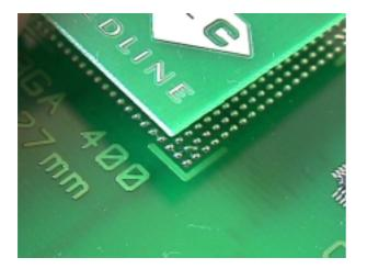
When all the terminations have reflowed and this has been confirmed the BGA can be lifted off the board using a vacuum pickup tool.
