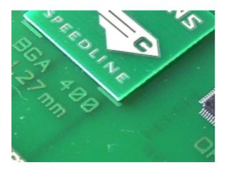
Shows the laminate BGA placed accurately using the BGA corner marks.
