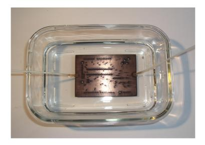
> After approx 5 minutes remove the PCB and rinse it under cold tap water for a few seconds.
