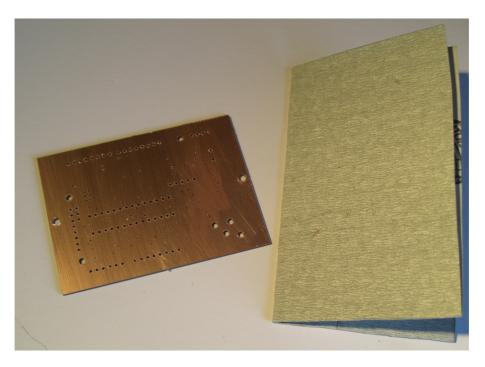
Rinse the board in cold tap water and make sure no debris is left in the holes. Blow the holes clear with compressed air if required.
