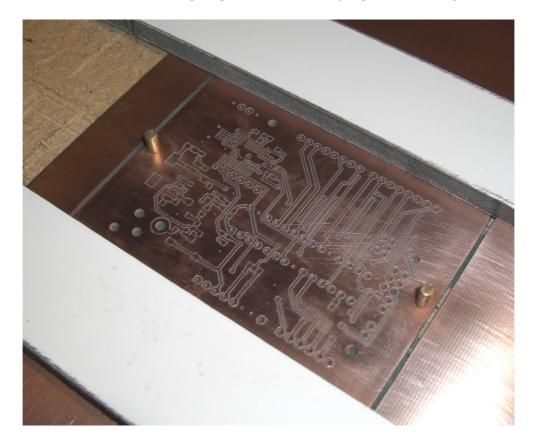
Below is a close-up view of the PCB's isolated tracks and the final board outline. Notice the small tab in the cut-out so that the board stays in place while it is milled:
