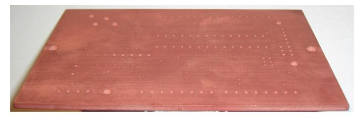
The image below is a close-up of some of the plated through holes after a few hours in the electroless copper plating bath:
