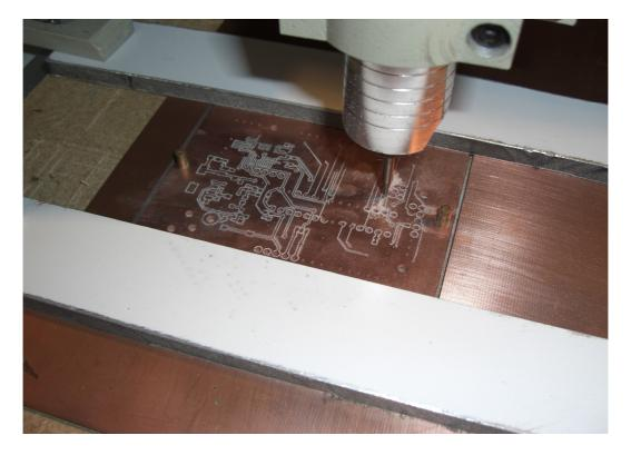
The image below is the board once all the tracks have been isolated. And is ready to be cut out of its matrix (extra board used for the aligning holes and clamping mechanism):
