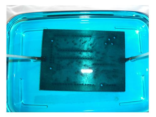
The container used in the above picture contained 200ml of electroless copper plating solution, therefore 2.0ml of 37% aqueous formaldehyde was used.
