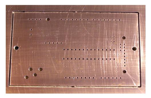
A freshly drilled PCB may look clean, however, it must be chemically clean for good adsorption of the metallic atoms and subsequent plating. Any grease produced as a by-product of the drilling must be removed from the holes and the surface of the copper must be mechanically cleaned so that it is free from oxidation. It cannot be emphasised enough how important the board cleaning process is, so be patient and vigilant when performing the task.
