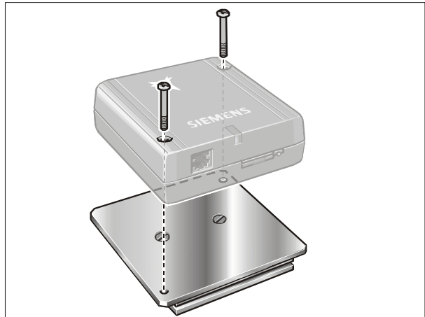
Figure 12: Attaching MC35i Terminal to a top-hat rail
