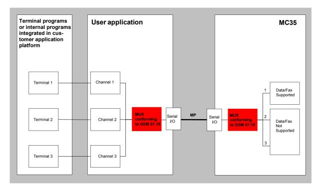
To make the three virtual interfaces (channels) available, both the MC35 module and the user application must contain MUX components which communicate over the Multiplexer Protocol. In the MC35 module, the MUX/MP software is already incorporated. The user application should either integrate the MC35 MUX/MP software or include a MUX/MP developed by the customer.
