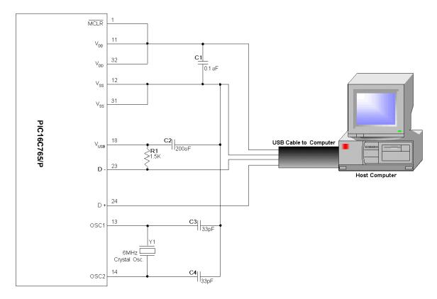
Note: Be sure to pull D- up to  $V_{USB}$  (via R1) *not*  $V_{DD}$ . For more on why this is done see the section Universal Serial Bus:Transceiver:Regulator in the PIC16C745/65 datasheet.
