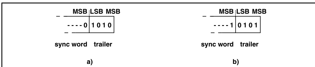
Figure 6.6: Trailer in CAC when MSB of sync word is 0 (a), and when MSB of sync word is 1 (b).
