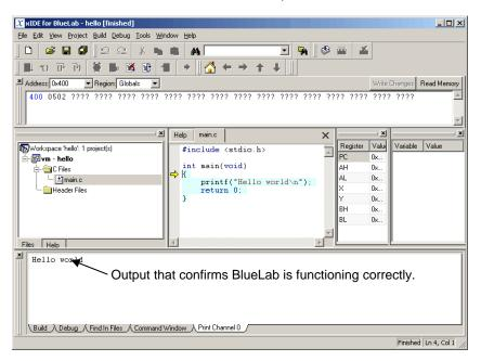
The output 'Hello world' confirms that the BlueLab software has been installed and is working correctly.
