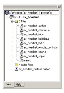
The file structure can be navigated and files opened in the text editor by double clicking on a file.
