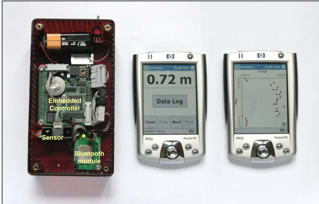
Figure 5 – Data logging embedded system using the FlexiPanel protocol to create user interfaces on Pocket PCs.
