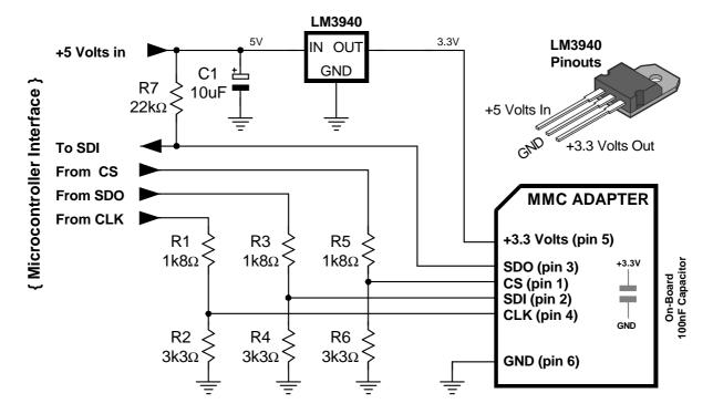
The LM3940 Low Dropout Regulator efficiently reduces the voltage from 5 Volts to 3.3 Volts. However, we still have the problem that the PICmicro<sup>tm</sup> will output 5 Volts from each of its pins when set high, placing the MMC card under stress, so simple resistor dividers are used to drop the voltage to a safe level before entering the card.
