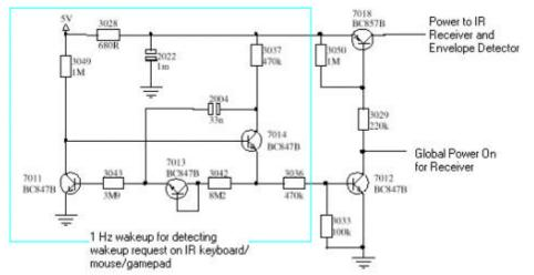
This is a -Hz oscillator with an on-time of around 20%, which gives power to the IR receiver. When the microcontroller is working this oscillator is frozen to give constant power to the receiver.
