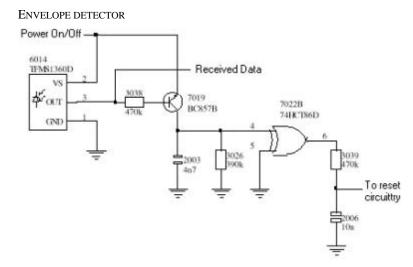
Integrates the receiver pulses and makes a reset of the microcontroller. Under normal working conditions, this part of the circuitry remains dormant. The device kicks into action only after it is put into suspend. It will be enabled every 1 second to scan for any IR signals from the remote IR keyboard/mouse/gamepad.
