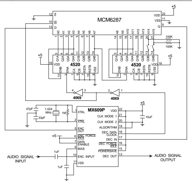
Figure 1: Audio Delay Circuit
