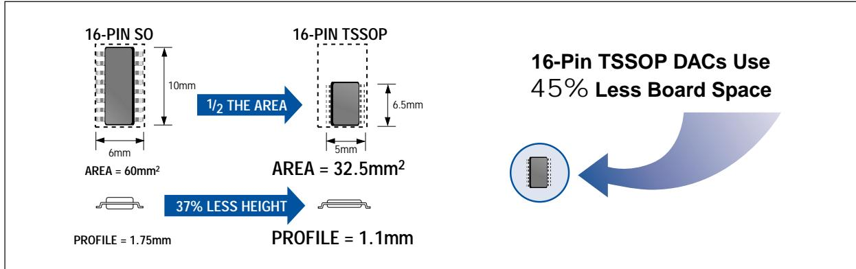
Maxim now offers an 8-bit, single-channel, current-output DAC (MX7524) and an 8-bit, triple-channel, voltage-output DAC (MAX512) in tiny TSSOP packages. The TSSOP package reduces thickness and footprint by as much as 45%.
