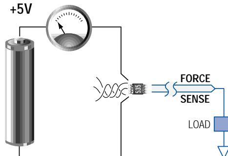
The MAX535 is the smallest, lowest power 13-bit voltage-output DAC available. The device operates from a single +5V supply and draws only 300μA of current (excluding the reference current). Several features make it ideal for industrial and instrumentation applications, including a space-saving 8-pin μMAX package, a rail-to-rail output, and a power-on reset function that resets the DAC output to 0V.
