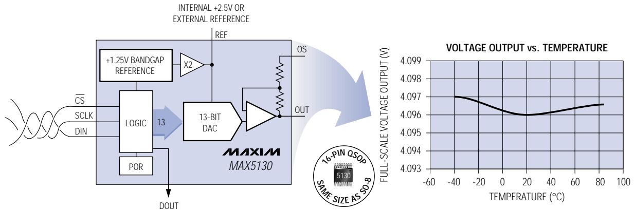
**Choose from 12- or 13-Bit Resolution, 3V or 5V Supply, and Voltage Out or Force/Sense Versions**
