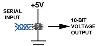
For general-purpose 10-bit applications, the +5V MAX5354 and the +3.3V MAX5355 single voltage-output DACs provide true 10-bit accuracy ( $\pm 1\text{LSB}$  INL and DNL) while using the least amount of board space—0.02in<sup>2</sup>. Features include power-on reset, a 10μs settling time, and a rail-to-rail output swing.
