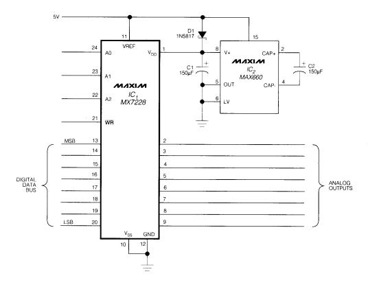
Figure 1. Because a voltage-doubler charge-pump IC supplies 10V to the octal D/A converters' references, the converter outputs can range from rail to rail (0 to 5V) of the applied supply voltage.
