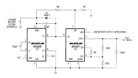
Figure 1. Operating without magnetic components, this circuit derives a regulated 5V from a 3V lithium battery and delivers load currents as high as 100mA.
